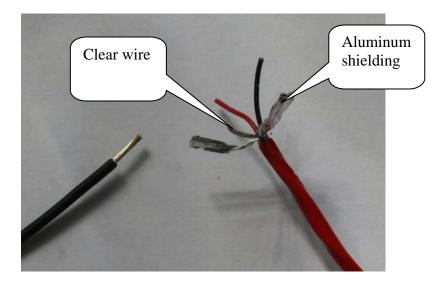
Cut the <u>aluminum shielding</u> and the <u>clear wire</u> off. Cut them back to where the red wire jacket ends.
