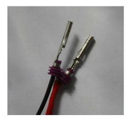
The red wire must go into connector location "A" and the black wire into "B". The connector provided with the speed sensor will snap into the BS3 driveshaft speed sensor harness connector.
