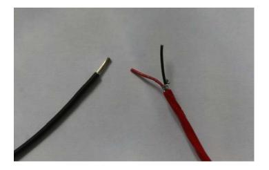
Strip <sup>3</sup>/<sub>4</sub>" of the wire jacket off from both the red and black wires
