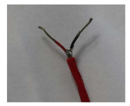
Twist the fine gauge black wire around the heavier guage black wire (with the eyelet at the other end).
