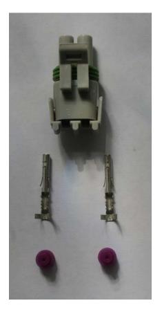
Black Wires - Slide the connector seal onto the black wires that are twisted together, and then securely crimp a female terminal onto the black wires.
