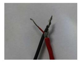
The next step is to crimp the female terminals from the Packard 2-way connector kit supplied with the sensor, onto the wires, see below.
